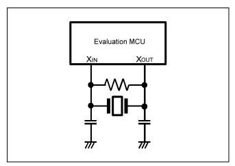
Figure 2.9 Circuit in which oscillation does not occur
